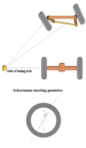
Caster angle  $\theta$  indicates kingpinpivot line and gray area indicates vehicle's tire with the wheel moving from right to left. A positive caster angle aids in directional stability, as the wheel tends to trail, but a large angle makes steering more difficult.
